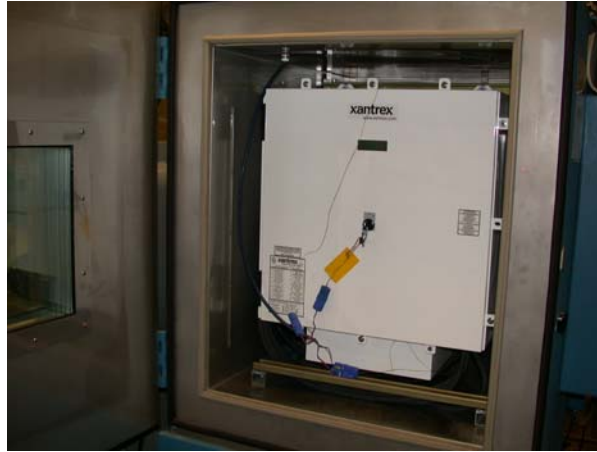
Figure 2. PV20208 inside temperature chamber
